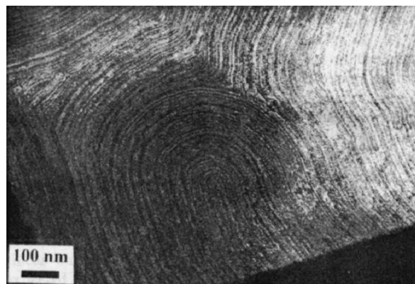
Figure 27. TEM image of the channel pattern for a sample of mesoporous film grown at the boundary between air and water showing a curved mesopore arrangement created due to constraints on packing in the film [151]. Reprinted with permission from J. mater. Chem. , 1997, 7, 1755.
